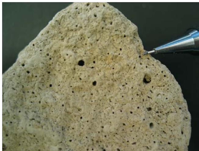
FIGURE 5. The porosity created in a clay soil as a result of micro-fracturing (the cross bedded striations and large holes from steam pressure)..
